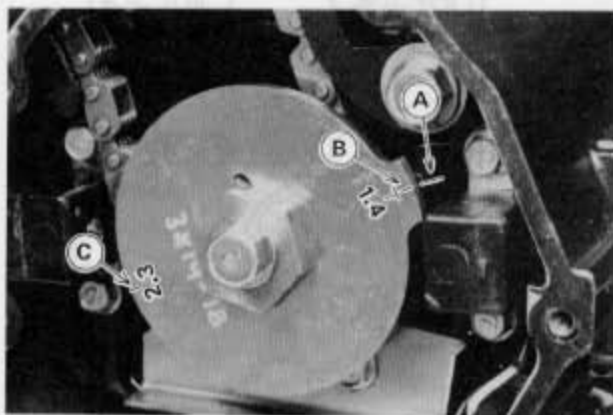
A. Timing Mark B. TDC mark for #1 and #4 pistons C. TDC mark for #2 and #3 pistons
