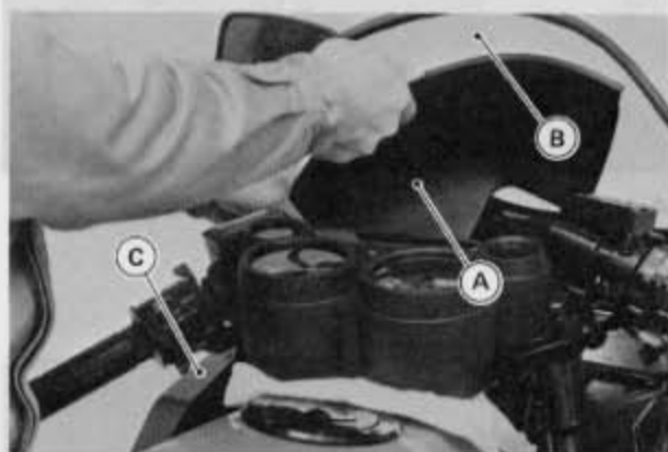
A. Inner Fairing half B. Windshield C. Upper Fairing
