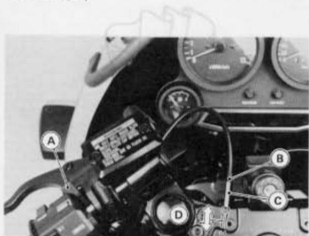
A. Choke Lever B. Locknut C. Adjusting Nut D. Play
