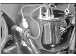
ABS Solenoid Valve Relay Fuse 15 A [A] ABS Motor Relay Fuse 25 A [B]
