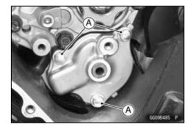
• Temporarily install the oil pump sprocket bolt [A].
