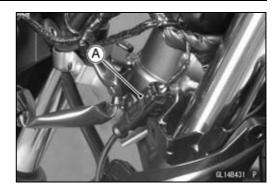
• Free the front wheel rotation sensor lead [A] from the clamps [B].
