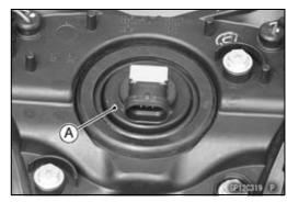
• Turn the headlight bulb [A] counterclockwise, and pull out it.
