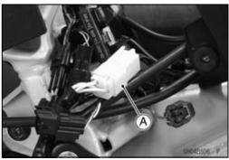
• Disconnect the neutral switch lead terminal [A].
