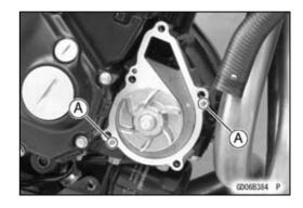
• Install the water pump cover and the bolts.
