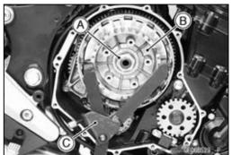
• Install the friction plates and steel plates, starting with a friction plate and alternating them.
