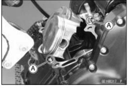
• The piston ring openings must be positioned as shown in the figure. The openings of the oil ring steel rails must be about  $30 \sim 40^{\circ}$  of angle from the opening of the top ring.
