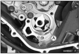
• Remove the oil pump cover [A].
