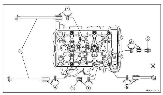
Apply a non-permanent locking agent to the M6 cylinder head bolts and M6 cylinder bolts [A], and tighten them.
