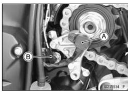
Oxygen Sensor [A] (Equipped Models)
