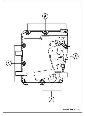
• Remove the following from the oil pan as necessary. Filter Plate Bolts [A] Filter Plate [B] Filter [C]
