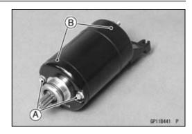
• Pull out the armature [A] out of the yoke [B].
