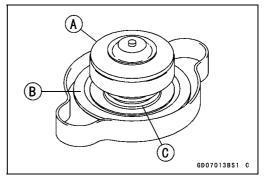
• Install the cap [A] on a cooling system pressure tester [B].
