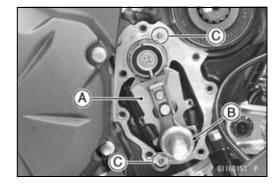
• When the new needle bearing [A] is installed in the shift shaft cover [B], press and insert the new needle bearing until it is bottomed.
