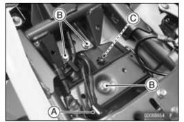
• Remove the following to separate the flap [A] from the reinforce [B].
