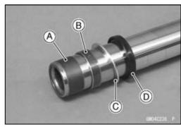
• Remove the cylinder base [A] from the bottom of the outer tube.
