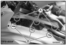
OWhile holding the portion [A], install the bolt [B] and washer.
