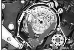
Remove: Clutch Hub [A] Spacer [B]
