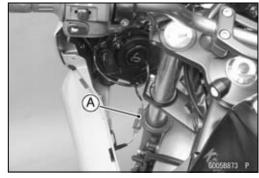
• Remove the quick rivets [A] from the lower fairings.
