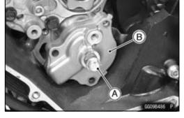
• Remove the outer rotor [A] for feed pump.
