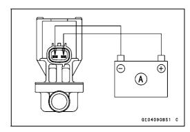
• Blow the air to the intake air duct [A], and make sure that the air does not flow through the outlet air duct [B].
