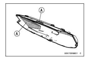
Olnstall the rear seat cover [A] so that the ribs [B] fit inside the rear fender [C].
