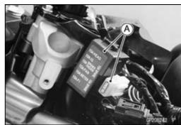
Pull out the fuses [A] straight out of the fuse box with needle nose pliers.
