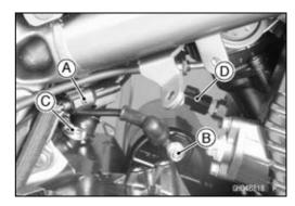
• Disconnect the alternator lead connector [A].
