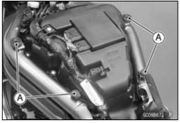
• Insert the fuel hose joint [A] straight onto the outlet pipe until the hose joint clicks.
