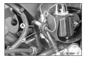
Remove the brake pipe joint nuts [A] with the flare nut wrench.
