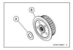
Install the washer so that the OUT SIDE mark [A] faces outward.
