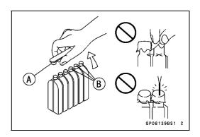
Place the electrolyte container upside down with the six sealed cells into the filler ports of the battery. Hold the container level, push down to break the seals of all six cells. You will see air bubbles rising into each cell as the ports fill.
