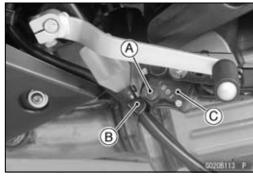
Remove: Spring [A] Sidestand Nut [B] Sidestand Bolt [C] Sidestand [D]
