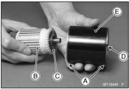
Align the marks [A] to assembly the yoke and the end covers [B].
