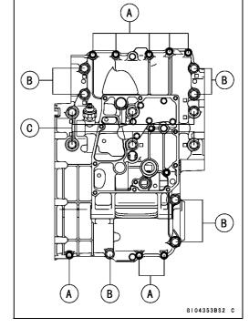
★ If the oil pipe is to be removed, follow the next procedure. OUnscrew the bolts [A] and remove the oil pipe [B].
