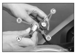
• Install the socket so that the projections [A] fit in the hollows [B] on the turn signal light.
