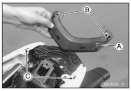
OFor other than US, CA and CAL models, install the grab rails and tighten the bolts.
