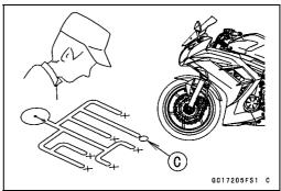
Even when the ABS is operating normally, the yellow ABS indicator light (LED) may go on under the conditions listed below. Turn the ignition switch to OFF to stop the yellow ABS indicator light (LED). If the motorcycle runs without erasing the service code, the yellow ABS indicator light (LED) may go on again.
