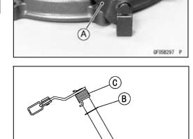
• Insert the release shaft [A] straight into the upper hole of the clutch cover [B].
