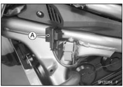
Connect one 12 V battery and turn signal lights as indicated in the figure, and count how may times the lights blink for one minute.
