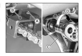
• Set the cutting and riveting pin [B] in the pin holder [A] as shown in the figure.
