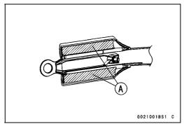
Olnstall the side cover so that the projection [A] fits into the grommet [B].
