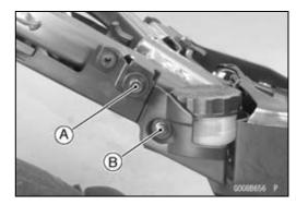
• Clear the hook [A] from the frame to remove the rear fender [B].
