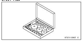
Steering Stem Bearing Driver,  $\phi$ 42.5: 57001-1344
