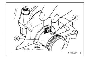
Crankshaft Main Bearing Insert/Journal Clearance Standard: 0.017 ~ 0.041 mm (0.0007 ~ 0.0016 in.) Service Limit: 0.07 mm (0.003 in.)
