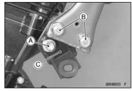
• Remove the rear engine mounting bolt and nut (upper) [A].
