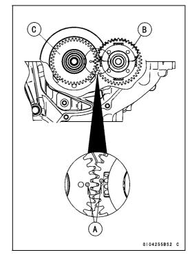
• Be sure to hang the camshaft chain [A] on the crankshaft.
