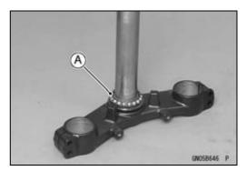
Remove the lower ball bearing inner race [A] (with its oil seal) which is pressed onto the steering stem with a suitable commercially available chisel [B].
