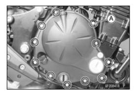
Turn the release lever [A] counterclockwise, and remove the clutch cover [B].
