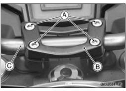
• Remove the lower handlebar holders [A] as necessary. ORemove:
