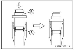
• Install the needle bearings [A], ball bearing [B] and oil seals [C] as shown.
