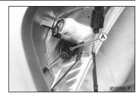
• Remove the bulb [A] from the socket [B]. OPush and turn the bulb counterclockwise.
