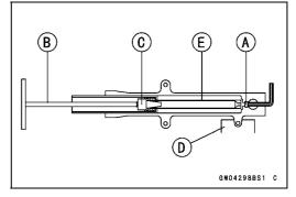
• Remove the cylinder unit [A], washer [B], and the spring [C] from the inner tube.
