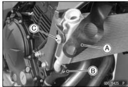
• Remove the radiator [A] by pulling it toward the left [B], noting the baffle plate [C] on the cylinder head cover.
