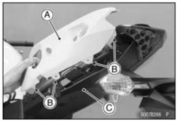
Olnstall the center seat cover [A] so that the projections [B] fit into the slots [C].
