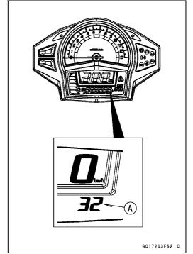
When the service code [A] is displayed, for first ask the rider about the conditions [B] of trouble, and then start to determine the cause [C] of problem.
