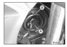
Release the hook [A] and remove the headlight bulb [B].
