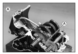
• Install the bearing [A] so that the positioning ring [B] fits into the bearing groove [C].
