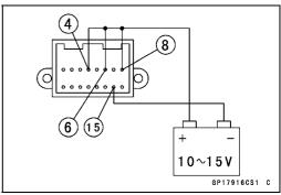
★If each light (LED) does not go on, replace the meter assembly.
